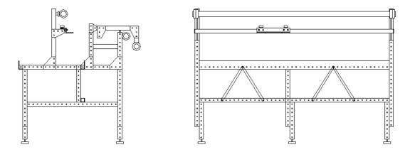
Step 6: Adjust the ruler bar height for adequate clearance from the bed of the quilting machine.
