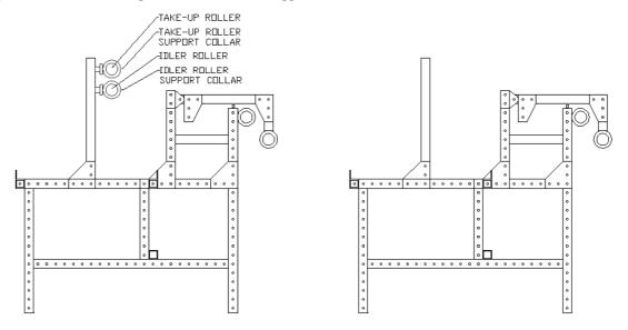
Step 2: Install the (2) ruler bar brackets on the slotted beams using (1) 5/16 x 3/4 Hex, (1) 5/16 lock washer and (1) 5/16 flat washer.
