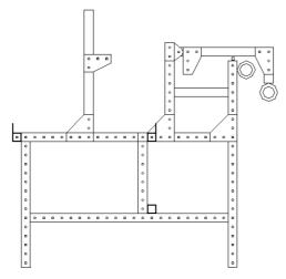
Step 3: Slide the ruler bracket onto the ruler bar as illustrated below.
