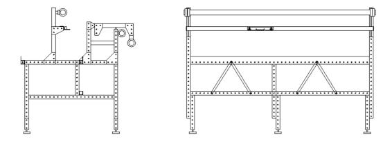
Step 6: Adjust the ruler bar height for adequate clearance from the bed of the quilting machine.
