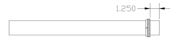
Step 13: Install the (3) rollers with gears into the roller end plates and make sure the gears on the rollers are facing the end plates with the gear assemblies. Install a roller collar onto the tube end and tighten the (3) set screws on the collar. NOTE: MAKE SURE TO LEAVE A SMALL GAP BETWEEN THE COLLAR AND THE PLASTIC BUSHING. THIS WILL HELP MAKE SURE THE ROLLER TURNS SMOOTHLY. CHECK ALL (3) ROLLERS TO INSURE THEY TURN SMOOTHLY. THEY SHOULD ONLY TURN ONE WAY.
