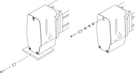
If you would like to install the mount onto the face plate, select the screw the laser mount will be installed on. NOTE: FOR ILLUSTRATION PURPOSES, THE INSTRUCTIONS INSTALL THE FRONT LASER MOUNT ON THE UPPER FACE PLATE SCREW.
