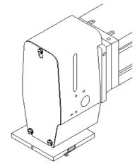
Step 5: Press the release lever and rotate the Innova head back to the normal position.
