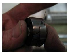
Remove the old bobbin and press in the new bobbin. Inset the bobbin making sure it turns clockwise when the thread is pulled (viewed from the bobbin side). Pull the loose thread up and under the guide into the case. Route the thread under the tension spring, and through the guide hole. Place the loose thread through the case slot.
