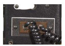
Step 2: Install the (2) double phone jacks provided in the PANTO VISION box into the encoder sockets on the back of the machine.
