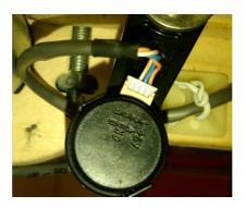
Step 2: Completely disconnect the original cables from the machine. Make sure to note where and how the cables are routed on the machine.
