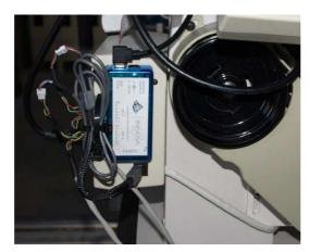
Step 5: Connect the original encoder cables to the blue Panto vision box plugs provided in the Tin Lizzie adapter kit. Reconnect the network plug of the original encoder cables to the rear of the Tin Lizze stitch regulator box.
