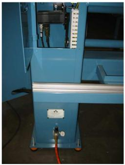
Figure 2.1 – Air Input location and Pressure adjustment
